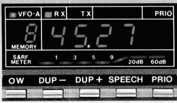
32 PL Frequencies. The IC-27A and IC-27H come complete with 32 PL frequencies ready to go and are controlled from the front panel knob. Each PL frequency may be selected by the main tuning knob and stored into memory for easy access along with frequency and offset.
